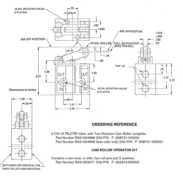
"A" Pilotair<sup>®</sup> Pneumatic Directional Control Valves Block Type Valves Three Way - Normally Closed
