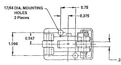
The Single-Direction Cam Roller Operator Kit assembled to the 2-MA-1A PILOTAIR Valve is designated the 2-CA-1C PILOTAIR Valve with Single-Direction Cam Roller.
