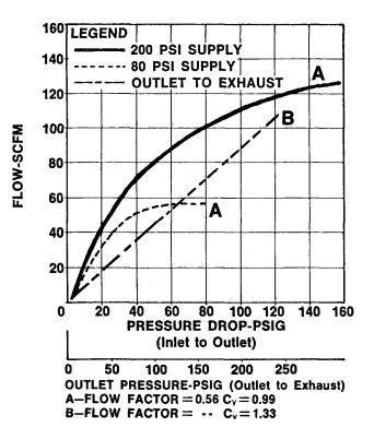
To determine flow from inlet to outlet for any pressure drop with 80 psi (5.5 bar) supply pressure, project up from the PRESSURE DROP Scale (permissible difference between inlet and outlet pressures) to the dotted curve.
