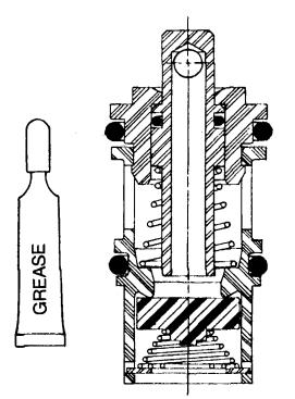
**CARTRIDGE REPAIR KIT** R431003743 (Old P/N P -055474-K0002) **"A" PILOTAIR VALVES CONTROLAIR VALVES** FLEXAIR VALVES, On-Off #3 Valve
