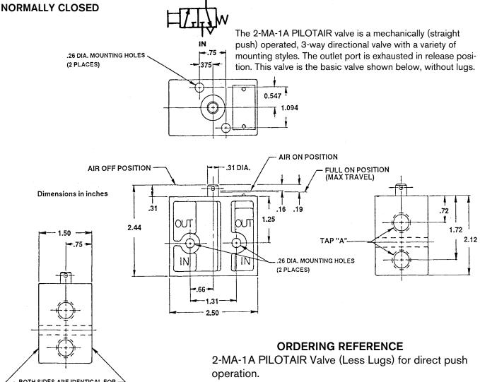
BOTH SIDES ARE IDENTICAL FOR **RIGHT OR LEFT HAND MOUNTING**  Part Number R431004659 (Old P/N P -058718-0000) "A" Pilotair<sup>®</sup> Pneumatic Directional Control Valves Block-Type Valves Three Way-Normally Closed
